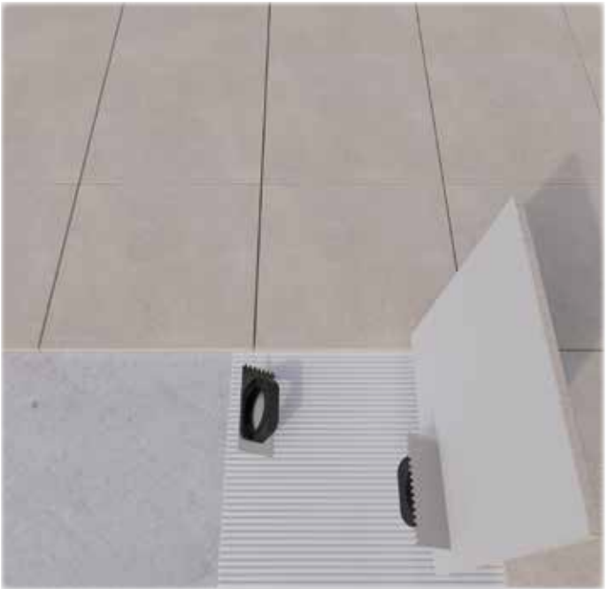
4- Thin-bed installation with cementitious adhesive Installation in terraces requires qualified personnel. It is only recommended to employ professionals with proven experience in this type of work.
