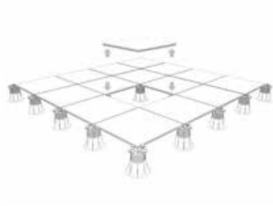
2. Panels can be lifted anytime, granting permanent access to the subfloor.
