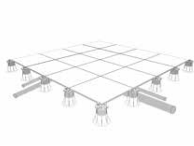
3. Elements such as pipes are completely hidden under the panels.
