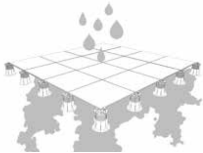
1. Optimal water drainage during rain or cleaning.
